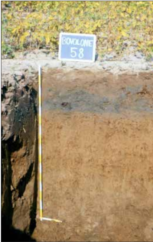
Plate 1: Soil of the Po Plain with compacted and hydromorphic subsurface horizon (plough pan).
