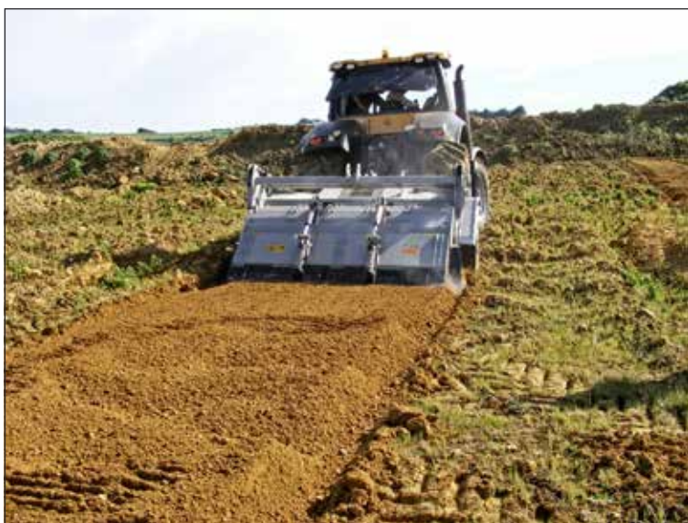
Plate 4: Rock chopping to increase soil depth can increase its vulnerability to both water and wind erosion.
