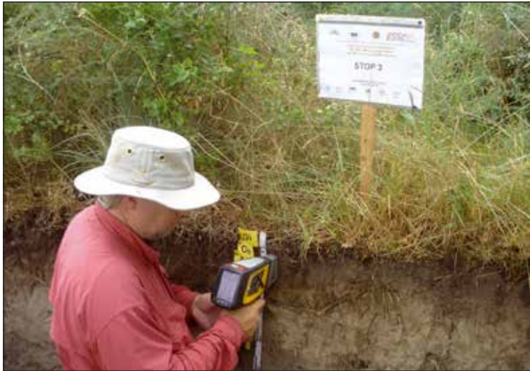
Plate 6. David Weindorf performing in-field XRF analysis on one of the soil profiles during the field trip.
