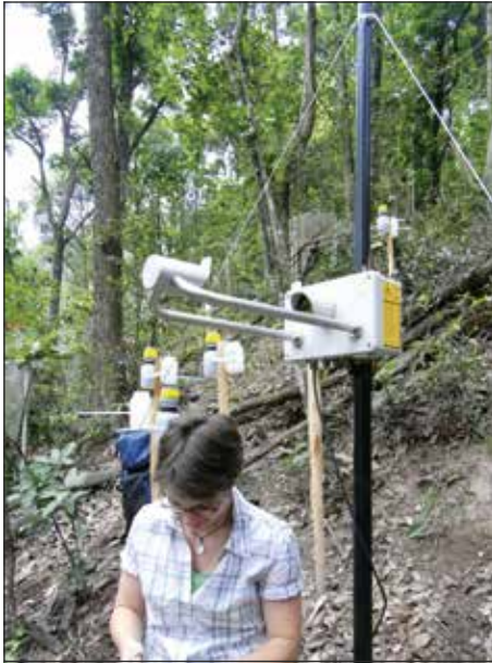
Plate 2: Laser disdrometer and array of splash cups and throughfall collectors in an 80-year old secondary forest at Gutianshan National Nature Reserve in Zhejiang Province, south-east China (photo taken 5 June 2010 by Christian Geißler).
