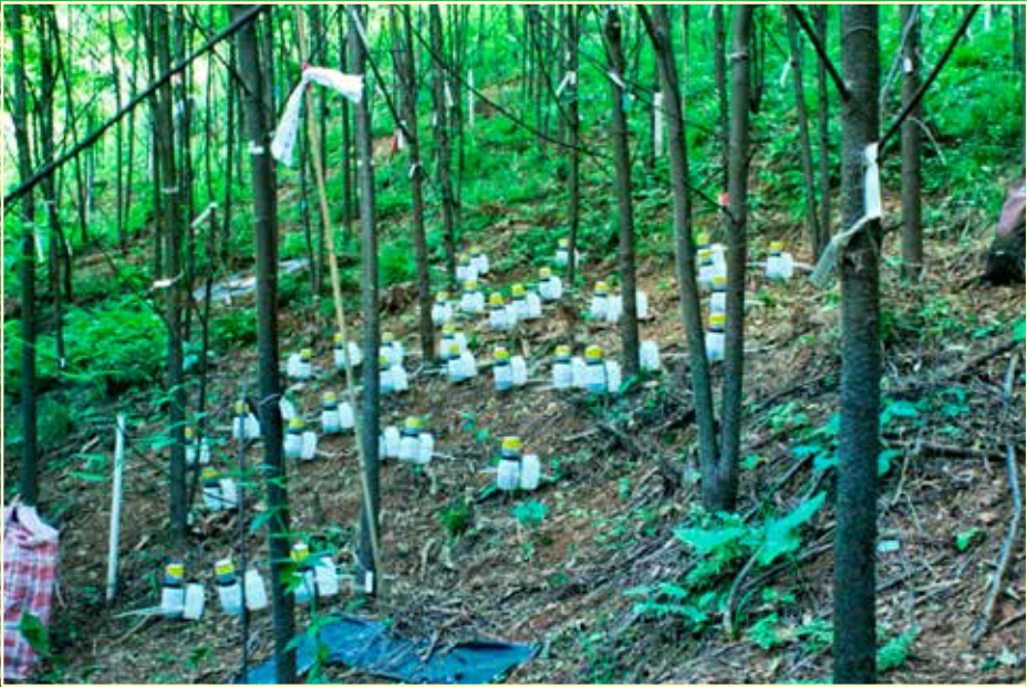
Array of splash cups and throughfall collectors under four year old trees in an experimental forest in Xinganshan, Jiangxi Province, south-east China. Photo taken 14 June 2012 by Philipp Goebes (Tübingen, Germany).
