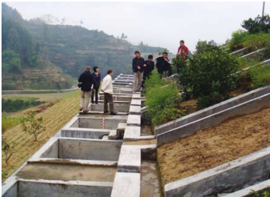
Wischmeier plots are being used in Zhigui, Hubei Province, China (October 2008) to study the effects of different kinds of terrace construction on erosion rates and processes.
