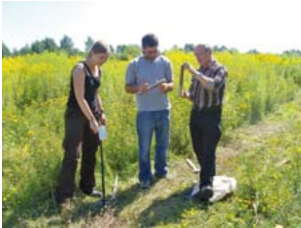
Soil magnetometry is the most effective field method for detection of magnetic iron minerals of both natural and anthropogenic origin occurring in topsoil.
